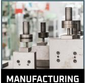
Coşkunöz will be leading the demonstration activities in the manufacturing sector. The coatings will be applied to stamping dies, which are precision tools used to cut and shape sheet metal into desired profiles. In addition to replacing the traditional hard chromium (HC) process, our focus is to increase the lifespan of the dies and explore the repairability of the MOZART coatings.
